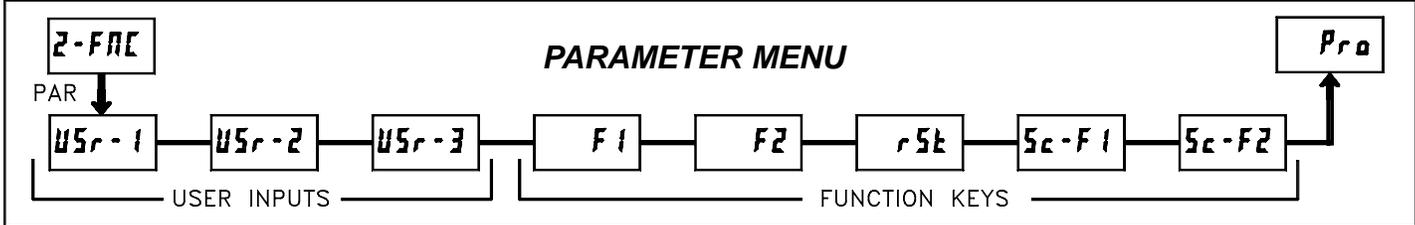
The three user inputs are individually programmable to perform specific meter control functions. While in the Display Mode or Program Mode, the function is executed the instant the user input transitions to the active state.
