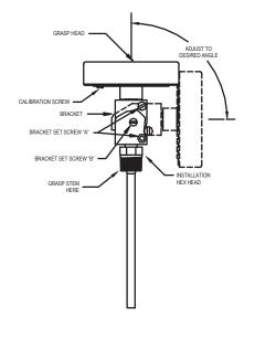
CAUTION: This thermometer is designed to allow the face to be positioned so that it can be easily read. REOTEMP Instrument Corp recommends that the thermometer be positioned only one time to assure proper performance during its lifetime.
