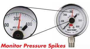
Spikes may only last for a fraction of a second but can do considerable damage.
