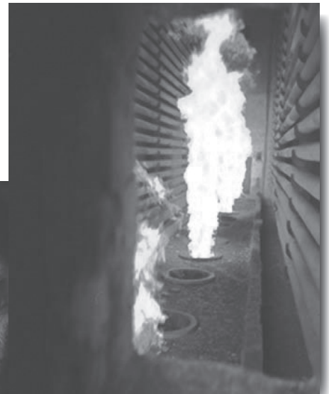
Gas Burner in Fire Box
