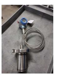
The diaphragm seal system was completely welded, including a weld of the fill port, for optimal performance in long-duration vacuum service. The system was filled with a high-temp, low pressure
