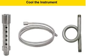
Heat is the slow killer of pressure instruments. Use cooling elements, capillaries, and standoffs, whenever possible.
