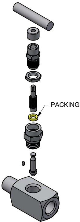
Packed Bonnet Seal Example
