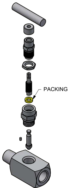
Packed Bonnet Seal Example
